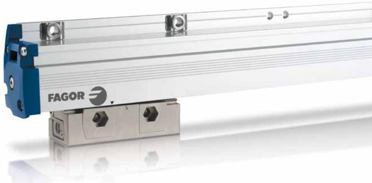
Linear encoder with small reader head, air intake and connector at both ends, with threaded head for different mounting options without the need for nuts.
